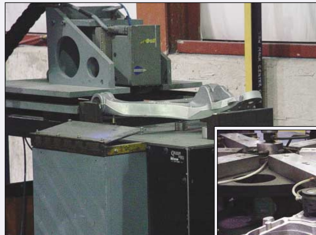
At Citation, PCRI and white light inspection proved to be 99.8% effective. In contrast, FPI and white light inspection were only 80% effective. In addition, the cost of PCRI was 33% of FPI.
