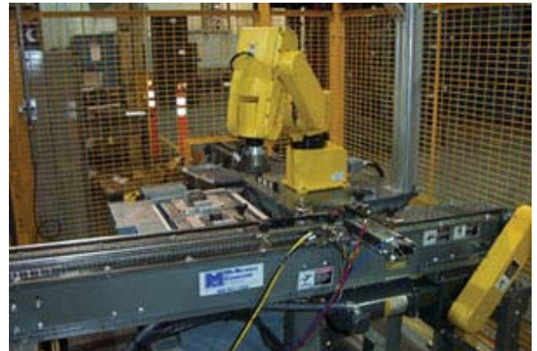
Quasar NDT system with robotic parts handling.
