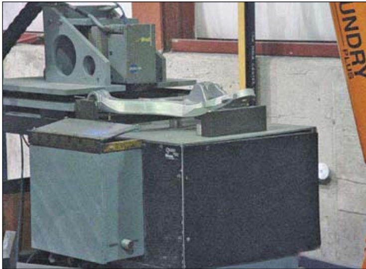
The front control arm is undergoing testing on the PCRT fixture at Citation Corp.
