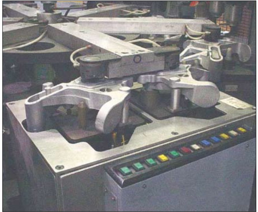
A rear knuckle is loaded onto the PCRT test fixture.
