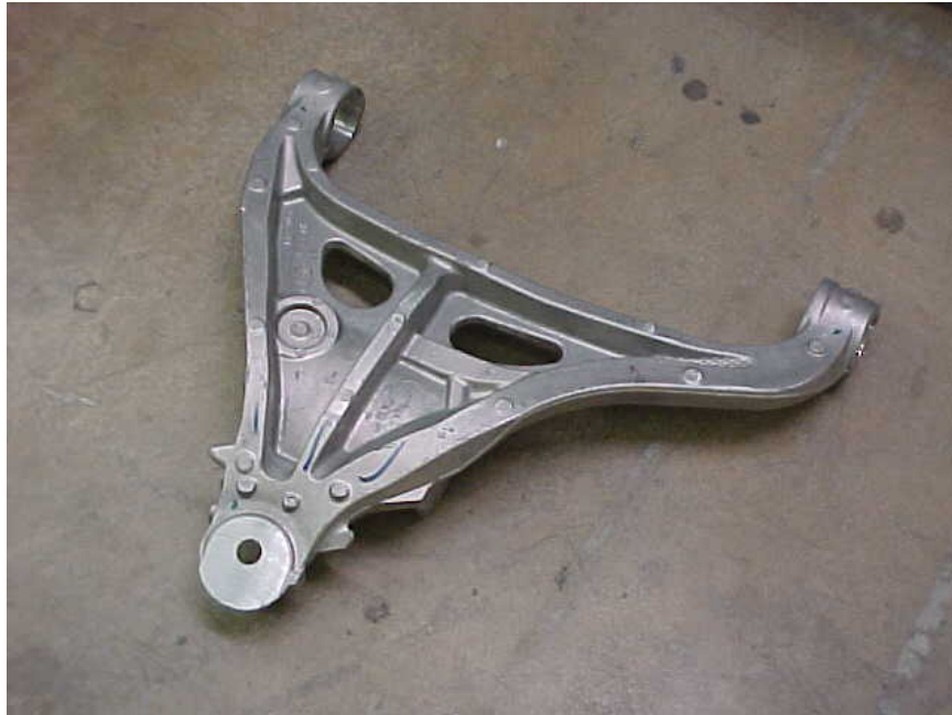
Fig. 1. The cast aluminum front control arm used in the PCRI application.
