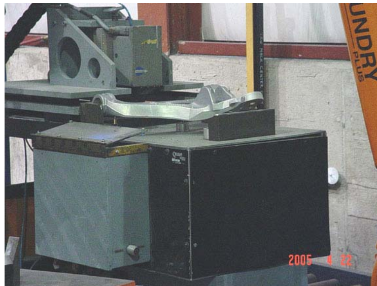
Fig. 5. The front control arm is shown under test on the PCRI test fixture.
