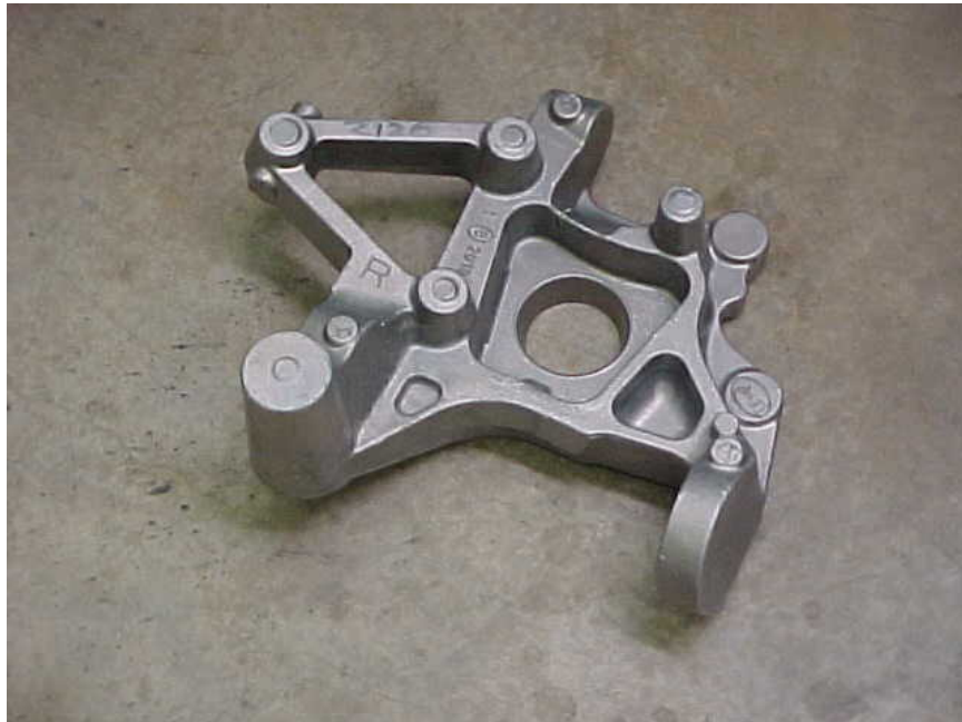
Fig. 2. The cast aluminum rear knuckle used in the PCRI application.
