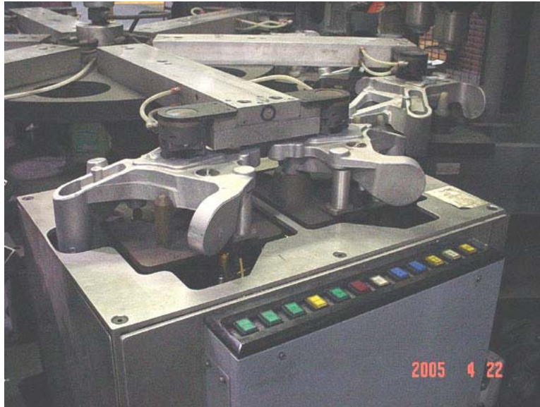
Fig. 6. A rear knuckle is shown being loaded onto the PCRI test fixture.
