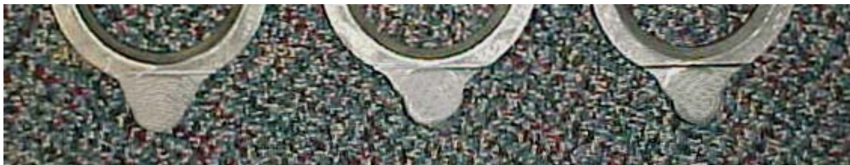
Figure 3. Three different cut depths used in the measurements increasing from left to right.
