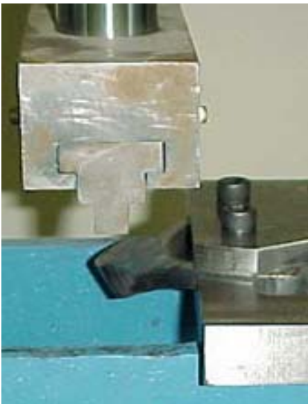
Figure 5. Test fixture for measuring Yield Force (bent clamp flange shown).
